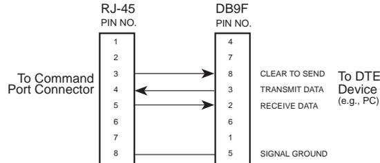
RJ-45 connector plugs into Command Port of TalkAnytime.
